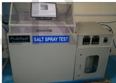
Fig 2: Salt spray testing equipment
