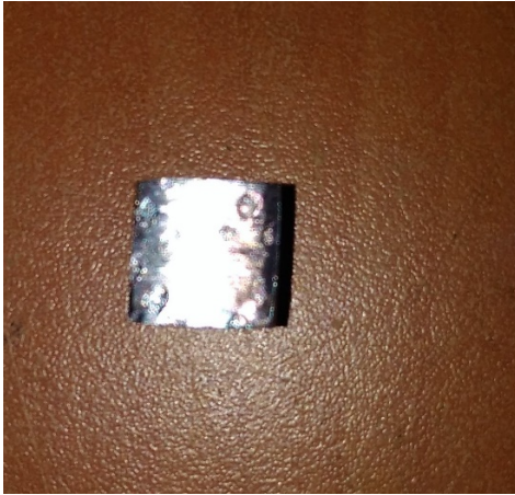
Fig 3: Coated specimen before rust formation
